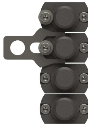
Main tool post of a CITIZEN K12/16E with SP-BS-31-00 + SP-BS-33-00 mounted on GSC-807 rotary tool holder
