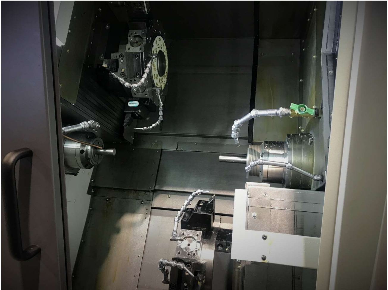
HECTO system mounted for tool cooling from turret disc
