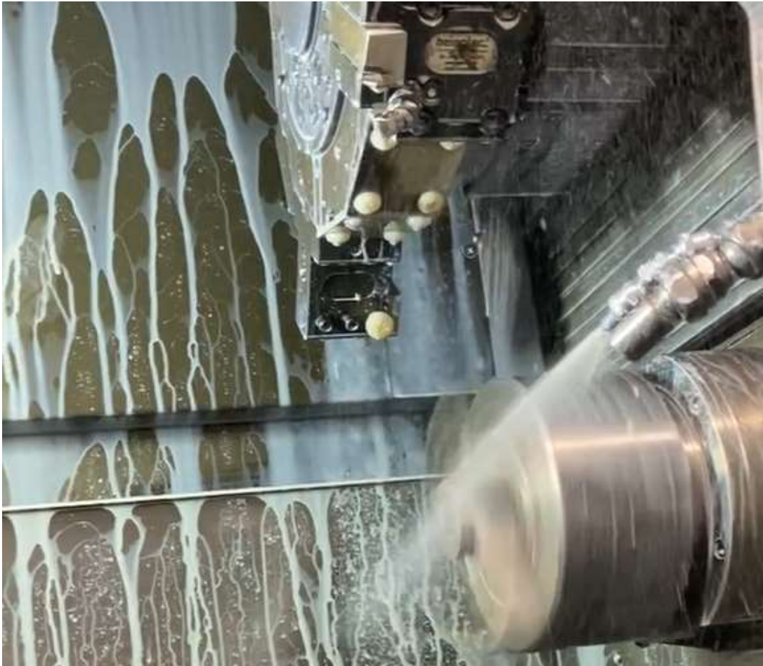
HECTO system mounted for air blasting of 2 jaw-chuck in sub spindle of CNC lathe before part transfer from main spindle.
