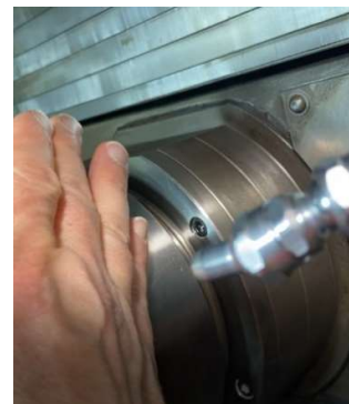
Perfect application for air blasting: no leaks thanks to "O" ring seals, even with the system not firmly fixed.
