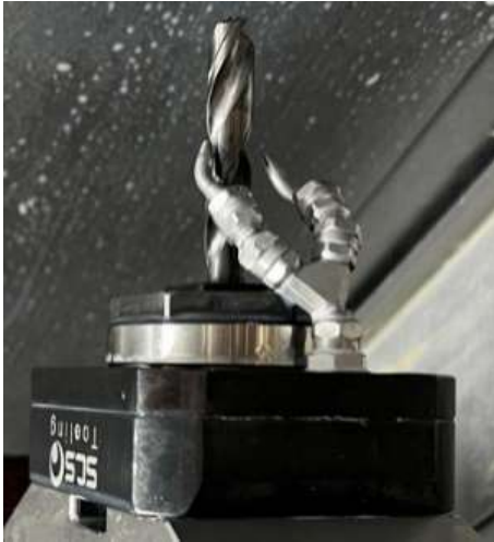
DECA system mounted in rotary tool holder 60° Distributor and 2 x Nozzle curved 45° ID:2 mm & L:20 mm
