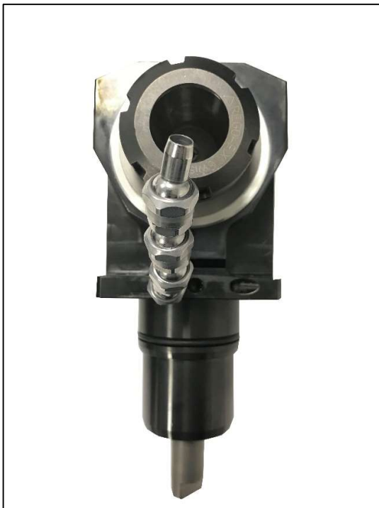
MK-TH-01-04 – Kit mounted in a rotary tool holder with 4 articulated segments, straight nozzle ID:6 mm and BSPP 1/8" connection.
